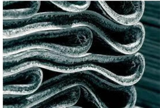
The extruder is switched on and pressures and temperature are monitored down the extruder barrel. The extruder head can have cooling water circulating to stop the rubber compound from curing in the head. The uncured rubber compound is generally supplied in wig-wag form in a continuous length. Alternatively it can be supplied as hide and manually cut into strips to feed the extruder.
