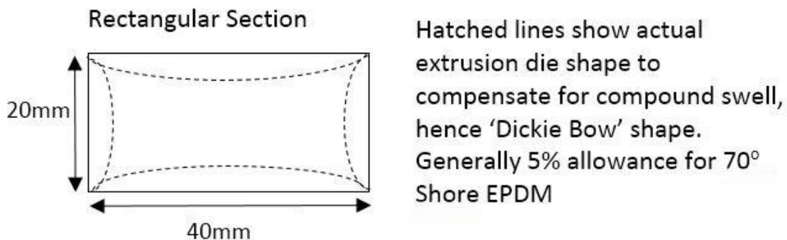
Dies for extruding thermoplastic profiles are generally cut oversize to that of the profile by around 10%. The profile is drawn down to size by the haul off.
