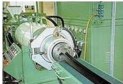
Now this is where the process can vary in the curing or the profile. When a rubber extrusion is produced the extrudate is un-cured i.e. it has not been vulcanised by heat treatment to create the cross linking of the polymer chains and thus create dimensional stability of the profile.
